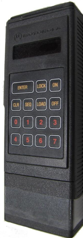
A DVP (Digital Voice Protection) code inverter by Motorola – used to provide secure voice communications over radio.
